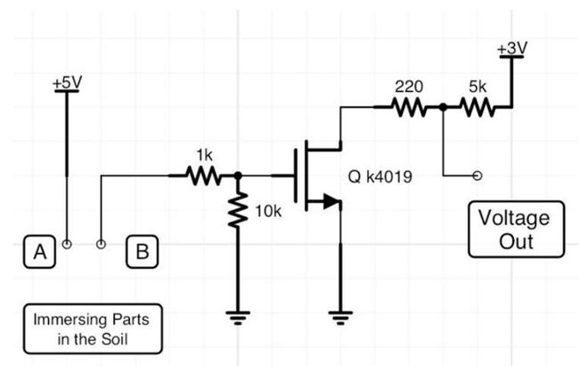
**Figure 1:** Circuit diagram of the impedance-based soil moisture sensor.
