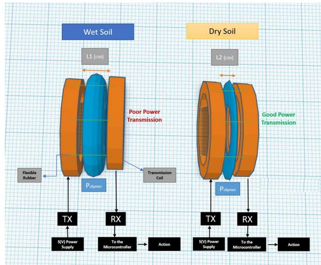
**Figure 2:** The 3D diagram illustrating the setup and operation of the polymer-based sensor. **Note:** Tx-Wireless Transmitter; Rx-Wireless Receiver.
