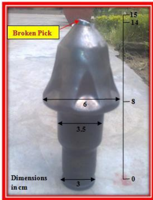
Figure 3. Broken pick due to overload.
