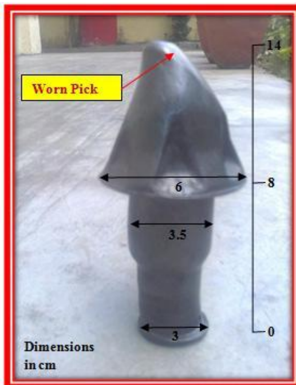
Figure 4. Worn pick due to rock abrasivity.
