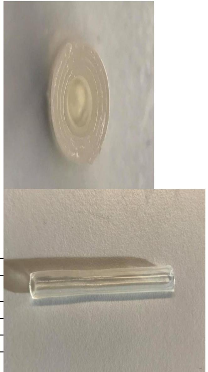
**Figure 1: Artificial alginate vessel.** The vessel was imaged immediately after fabrication with a simple dip-coating protocol, using 4.4% alginate solution and 200mM barium chloride, with the one base layer and 3 subsequent layer type (A) photographed along its axis (left) and the single 'subsequent' layer type (C) after removal from the dipping rod (right).
