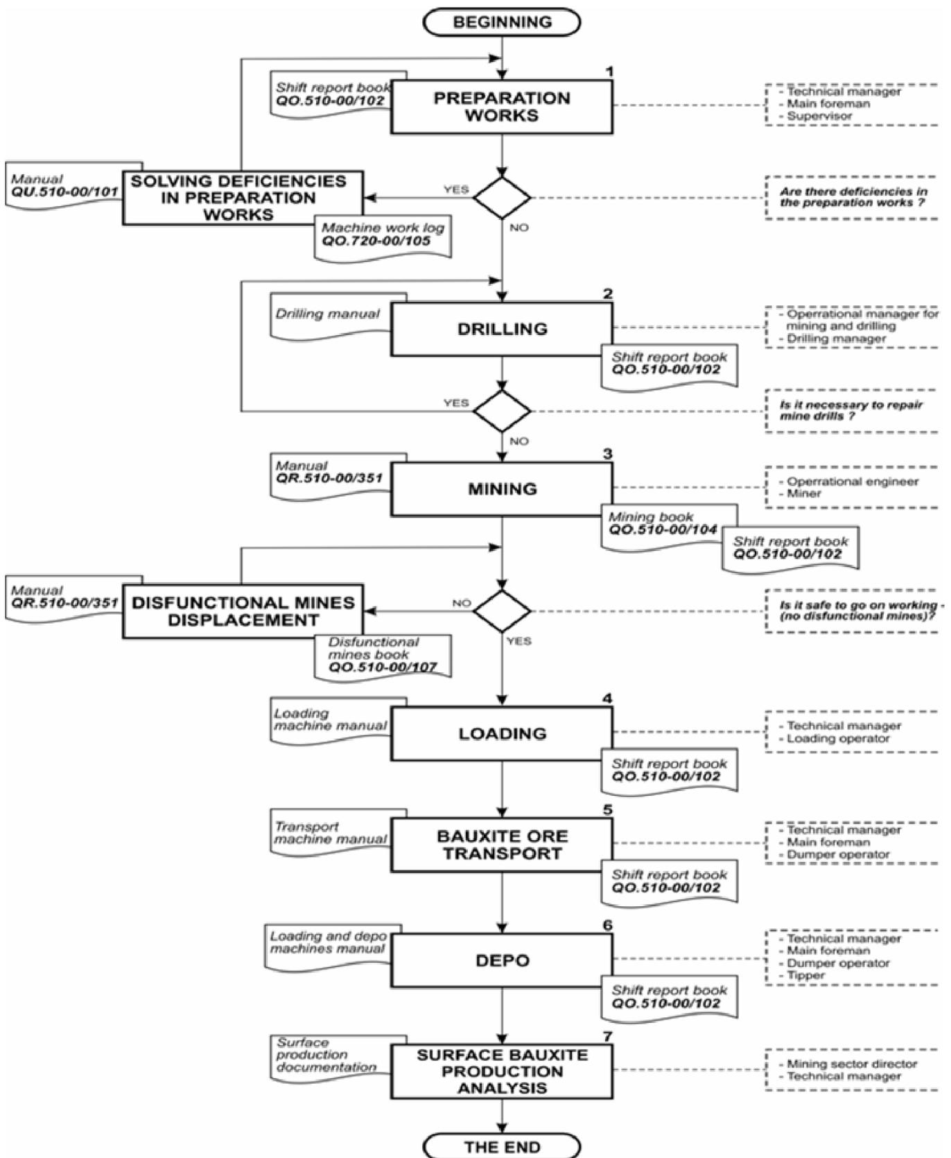
Figure 3. A flow diagram for bauxite surface-production process.
