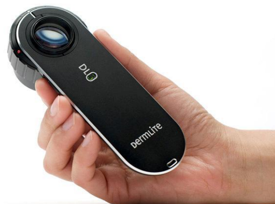
Figure 1. Recently developed product: "Dermlite III hybrid" allowing illumination in cross-polarized or non-polarized immersion fluid dermoscopy with optional cellular telephone photography (3Gen LLC).
