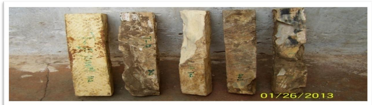
Plate 2: Obeche treated with Aguwa milk after exposure to termite
